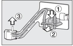
■ Press down on the small recess in the spout's holder (①) and pull the holder forwards and out (②). Loosen the milk pipework from its guides.
